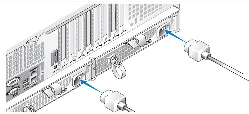
Connect the monitor's power cable to the monitor (optional). Connect the system's power cables to the system.
