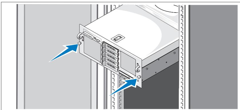
Install the system in the rack once you have read the “Safety Instructions” located in the rack installation documentation for your system.
